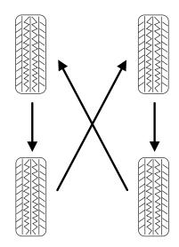
• Rear Wheel Drive (RWD) vehicles/Four Wheel Drive (4WD)/All Wheel Drive (AWD) vehicles (front tires at top of diagram)
